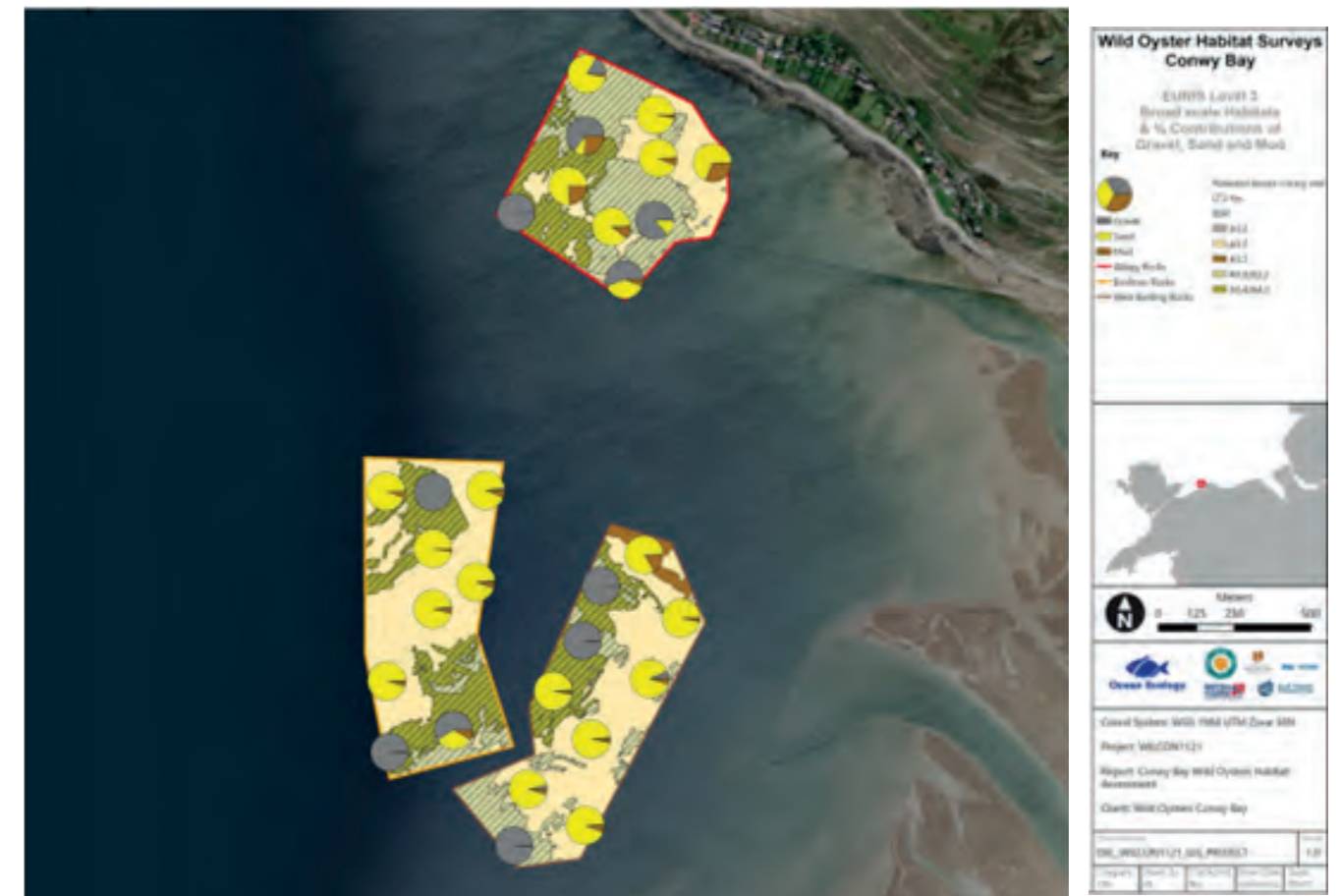
Figure 13. EUNIS Level 3 broadscale habitats based on geophysical and imagery data and sediment percentage contribution from grab samples across the survey area.
