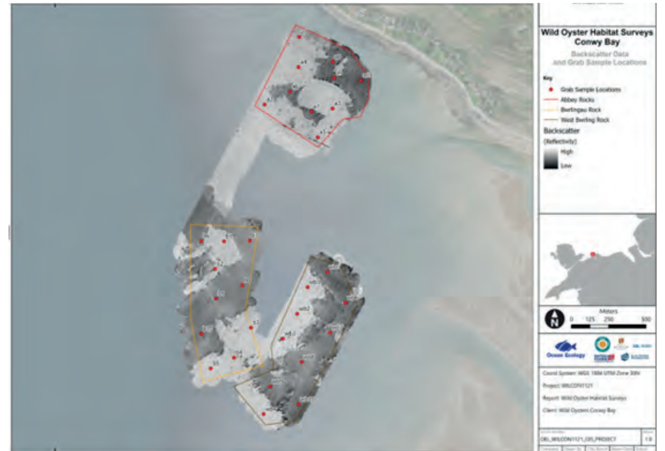
Figure 11. Overview of the Conwy Bay survey areas displaying the Backscatter and DDV/grab sampling locations. The backscatter data in this figure shows the substrate hardness across the three sites, with darker areas depicting softer ground and lighter areas the harder ground type.
