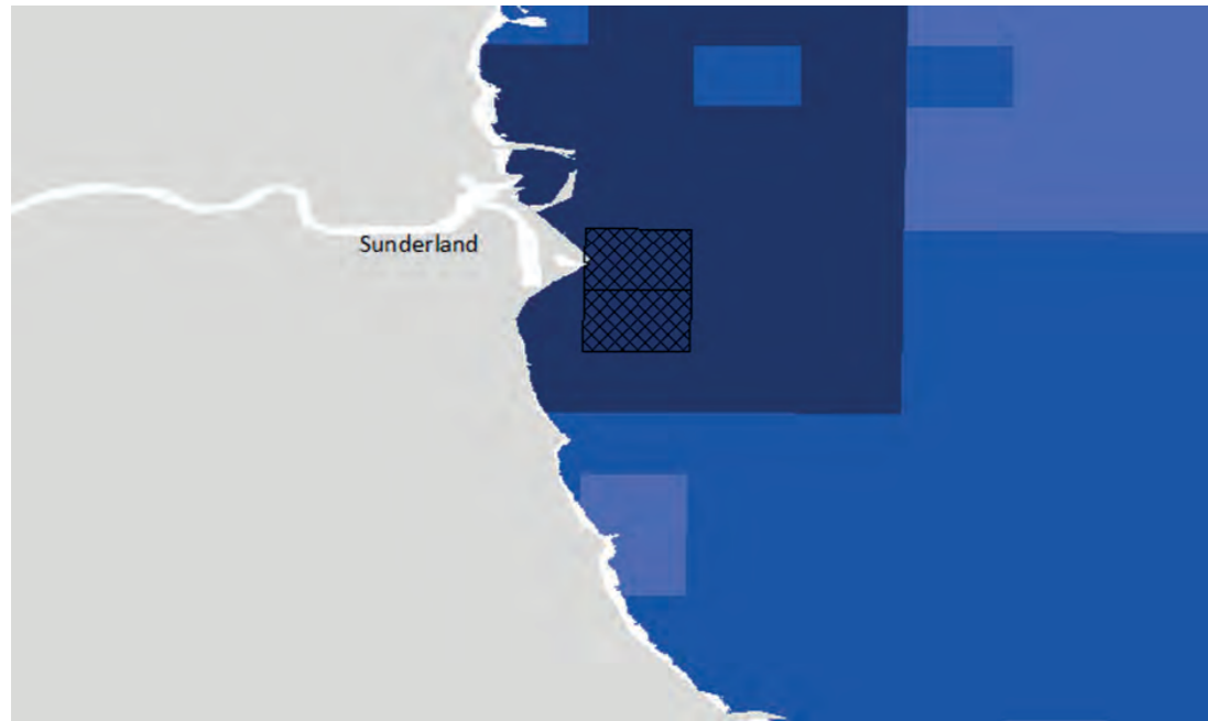
Site Suitability Model for the inshore area considered for the Tyne and Wear reef. Darker areas depict more favorable areas. This map is an amalgamation of the four parameters shown individually below (Shipwreck presence, substrate type, larval dispersal and vessel density). The hashed areas show the areas initially suggested but after further video analysis of the wider area, a new plot to the north (Figure 22 in the seabed report) was selected.
