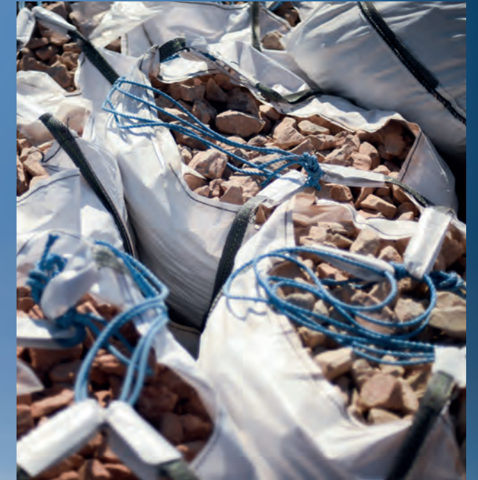
Main Photo: Loading of gravel cultch for the Conwy Bay reef. © Lucie Machin. Above: Limestone gravel cultch used to create the Conwy Bay reef. © Lucie Machin
